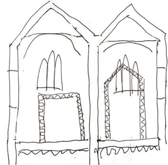
Thermal strategy 02: warm spaces within cool space, no changes to the external envelope
